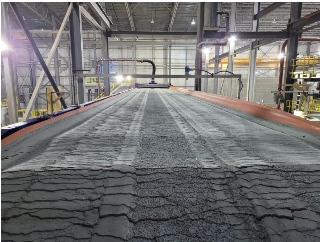
Spodumene concentrate on the NAL Complex filter press
