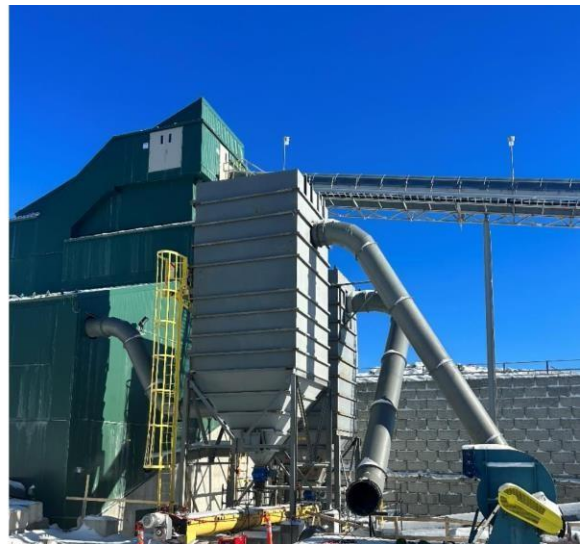
3 rd ore sorter chutes, conveyor, and feeder (left); dust collection system (right)
